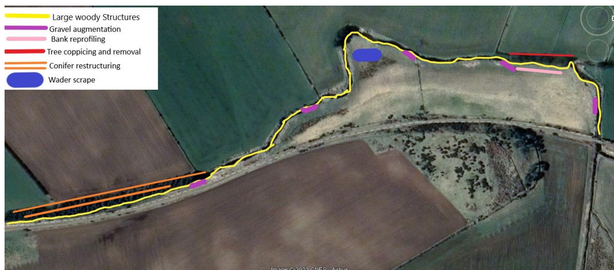
Figure 1. Example of habitat restoration proposal techniques, taken from Ebrie Burn Habitat Restoration Proposal 2024.
